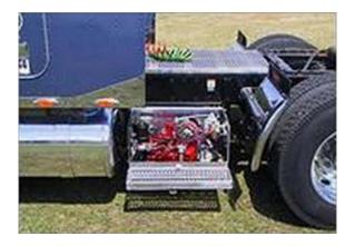
• *Battery or Alternative Powered* include heating and air conditioning systems that run off battery power, or a stored energy source. The battery powered units do not produce any emissions. However, they are expensive, heavy (additional batteries needed), and provide power as long as the battery is charged. The stored energy systems are fairly new to the market.
