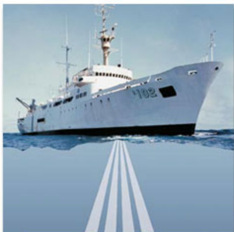
Figure 11. Diagrammatic beam arrangement of an Acoustic Doppler Current Profiler. Picture from RD Instruments web site, www.rdinstruments.com , reproduced with permission.
