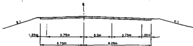
Figure 10. Recommended crowned section without median cable barrier being considered for use in Finland.
