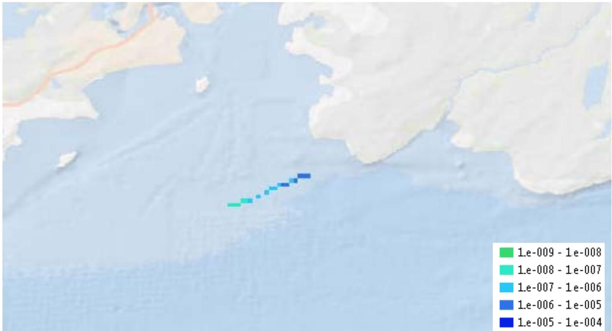
Figure 3-14: Aframax Anchorage Route Loss of Containment Frequency – Powered Grounding
