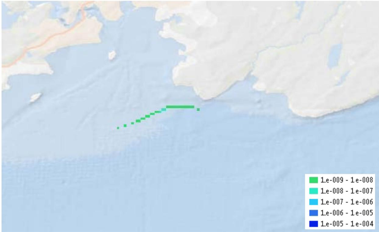
Figure 3-19: VLCC Anchorage Route Loss of Containment Frequency – Drift Grounding
