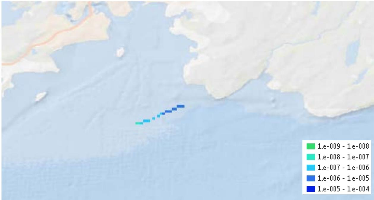
**Figure 3-15: Suezmax Anchorage Route Loss of Containment Frequency – Powered Grounding**
