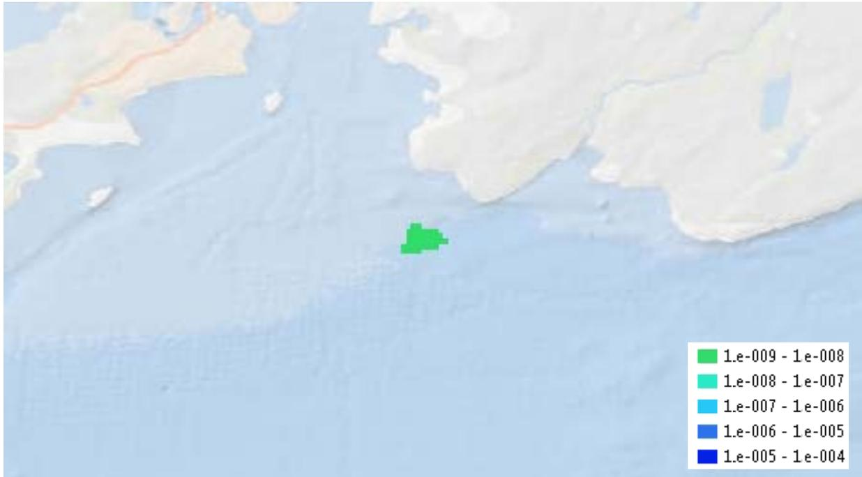
Figure 3-13: VLCC Anchorage Route Loss of Containment Frequency – Collision
