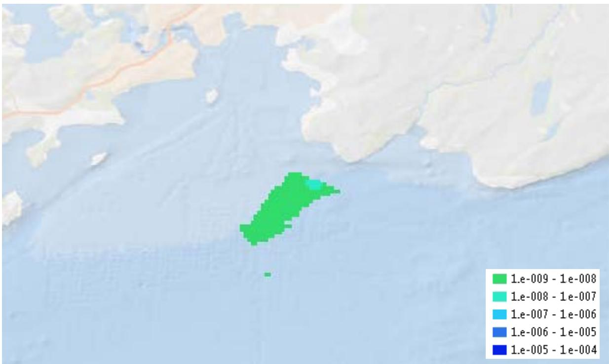
Figure 3-12: Suezmax Anchorage Route Loss of Containment Frequency – Collision
