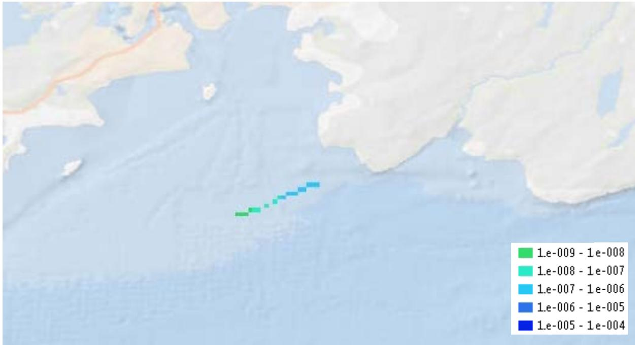
**Figure 3-16: VLCC Anchorage Route Loss of Containment Frequency – Powered Grounding**
