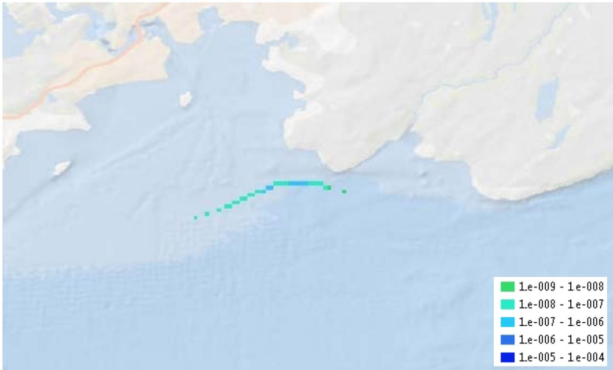
Figure 3-17: Aframax Anchorage Route Loss of Containment Frequency – Drift Grounding
