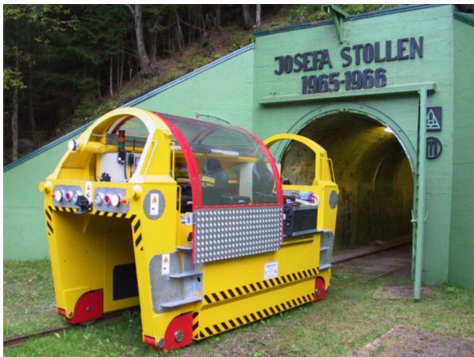
FIGURE 9-6 – VÉHICULE D'ACCÈS DU TAL (SOURCE –TAL)
