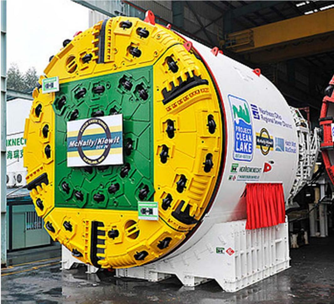
FIGURE 5-3 – TUNNELIER SIMPLE BLINDÉ EUCLID CREEK (DIAMÈTRE EXCAVÉ 8.2 M).
