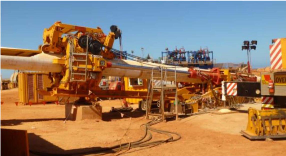
**FIGURE 6-9 – INSTALLATION D'UN PIPELINE DANS UN FORAGE EXISTANT PAR "PIPE THRUSTER" EN AUSTRALIE (PFEFF, 2014).**
