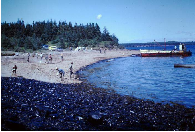
Figure 8.1. Testing the use of lime during shoreline clean-up of the Arrow spill. Image courtesy of Ed Owens.
