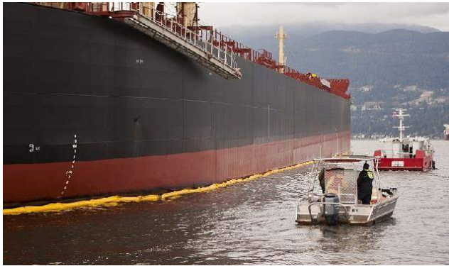
Figure 8.12 Booms placed around the Marathassa. Image from CCG (2015a) ( http://www.ccg-gcc.gc.ca/independent-review-Marathassa-oil-spill-ER-operation )
