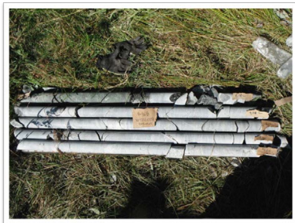
Figure 6: Carottage du roc au forage PO-16B
