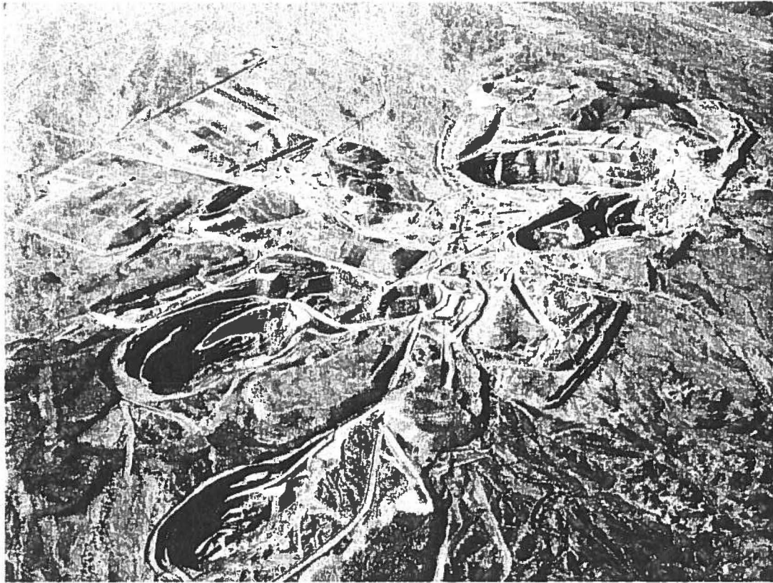
Figure 10. The active Mesquite Mine located about 52 miles northwest of Yuma, Arizona. Three pits, intervening waste dumps and a large cyanide leach pad is evident.
