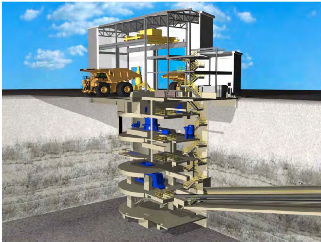
Figure 17.3 – Primary crusher, isometric view
