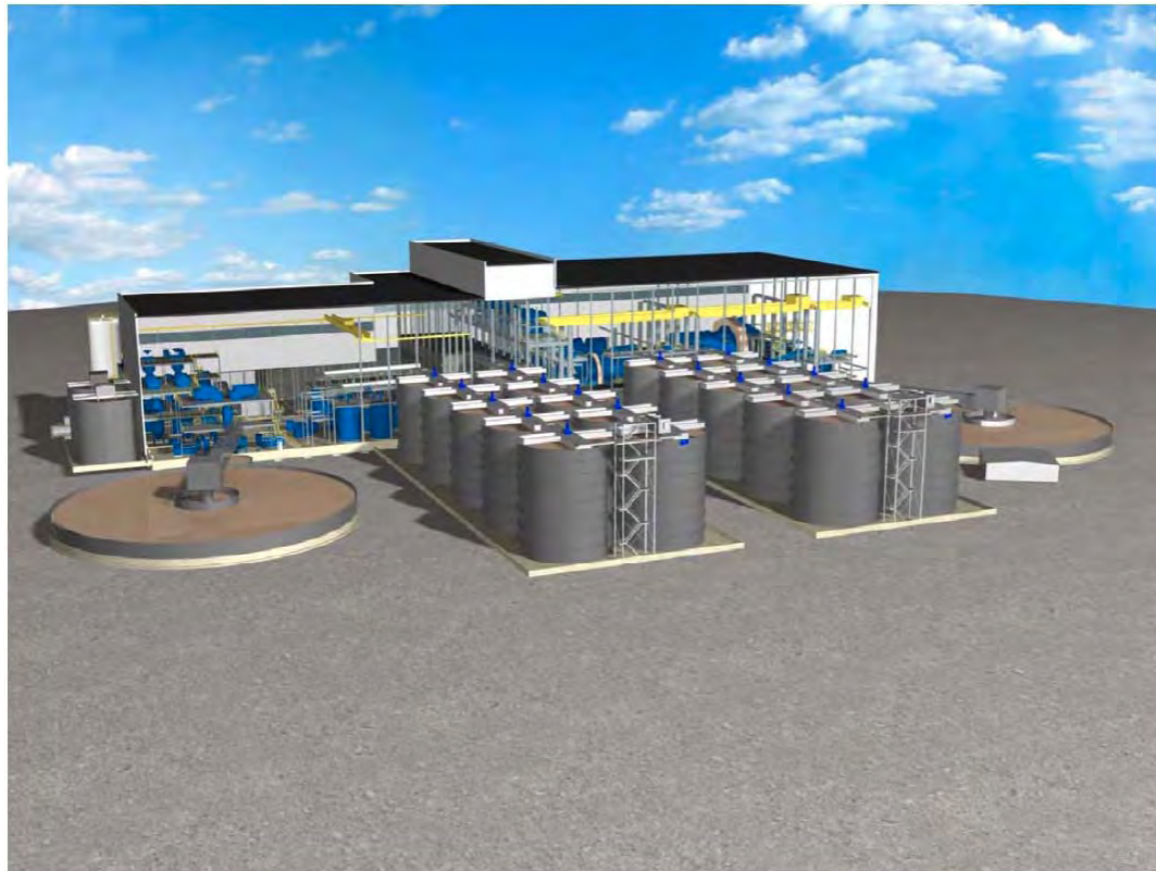
Figure 17.5 – Leaching circuit, isometric view
