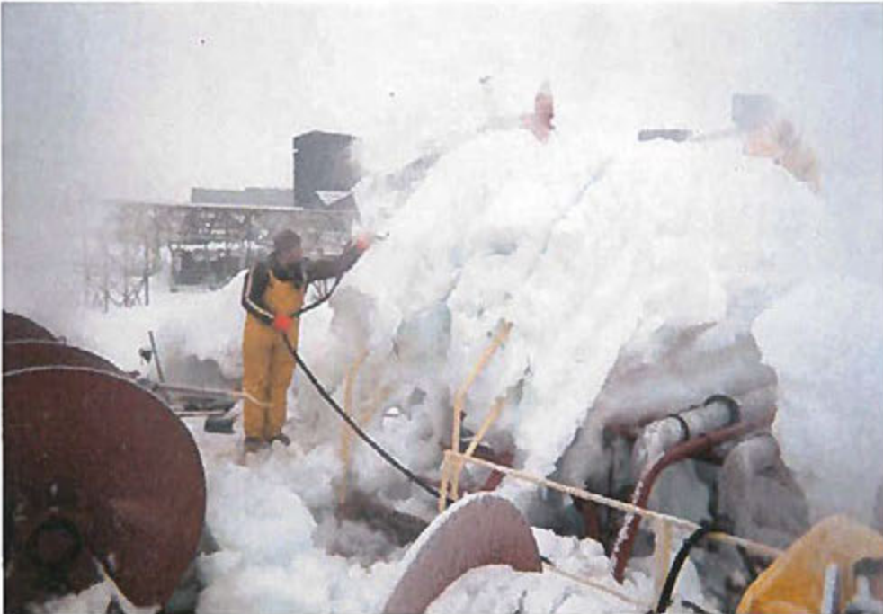
Figures 5.3J– Safe access to tanker bow fully obstructed by ice
