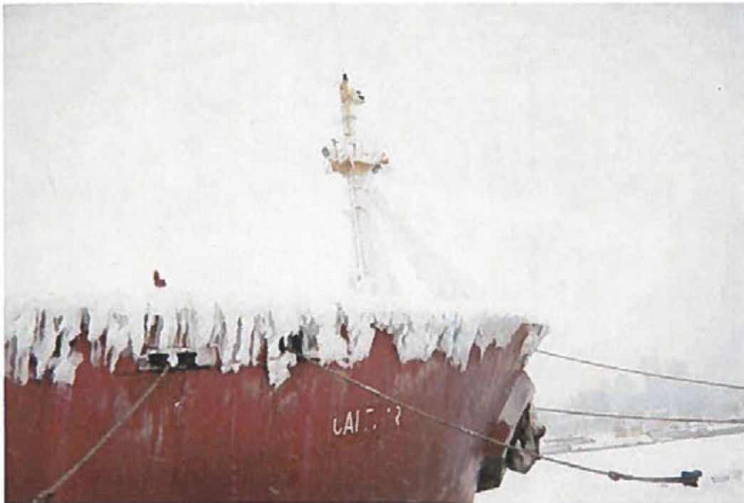
Figures 5.3A– Severe case of ice accretion in bow area
