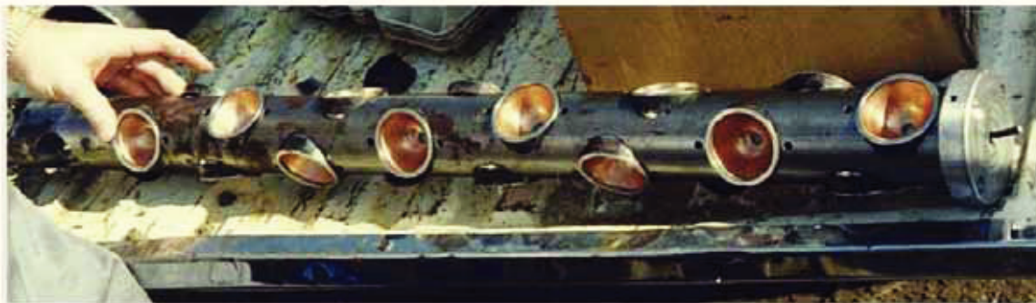
Figure 3-4 Canon à perforation
