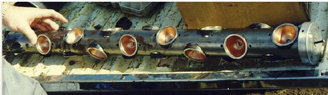
Figure 8 : Canon à perforation.
