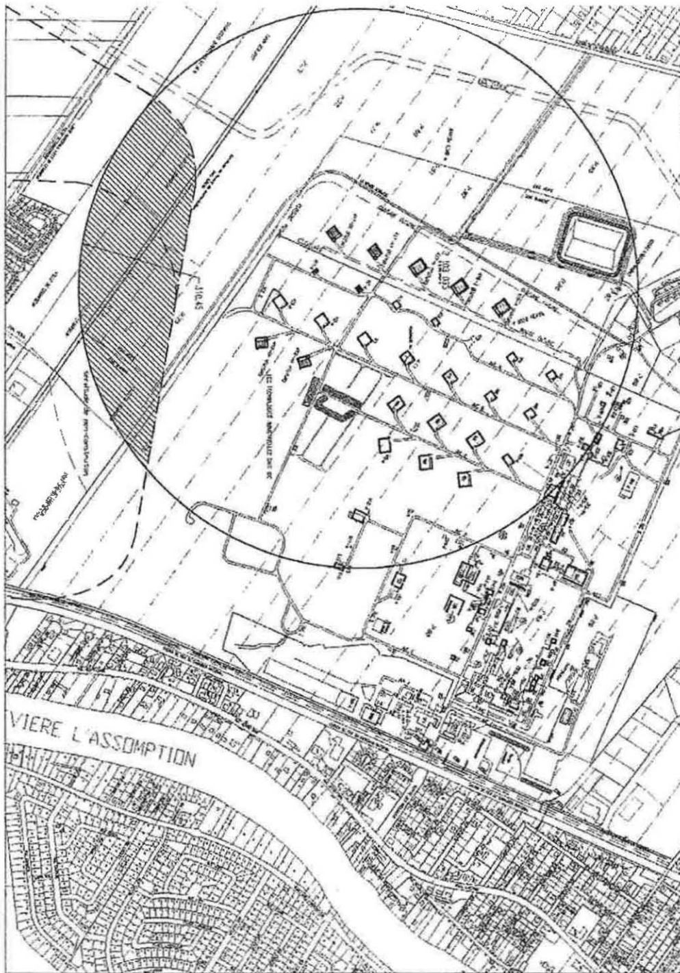
Figure 11. D7 Heavy Traffic PTR Separation Contour for Magazine 417-A
