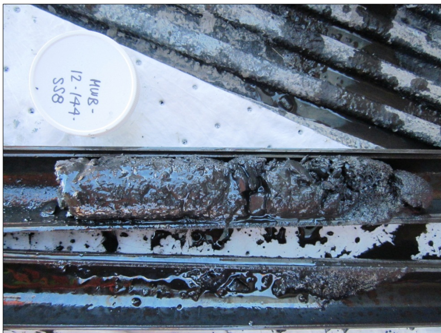
Photo 14: View of saturated soil sample MWB-12-144-SS-8 (4.5 m bgs), with evidence of free product.
