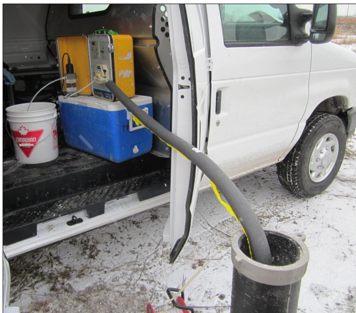
Photo 20: View of the low flow sampling set up for collecting groundwater samples.
