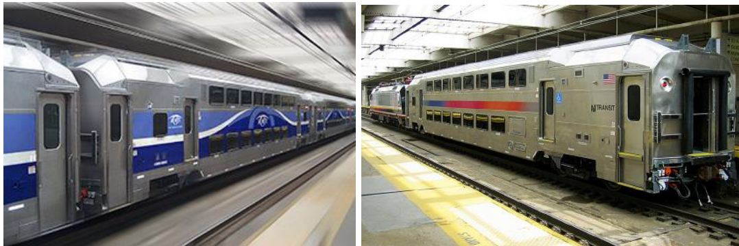
Left: AMT Bombardier multilevel car with high & low floor doors right: NJTransit Bombardier multilevel car with high & high/low floor doors (source: Bombardier)
