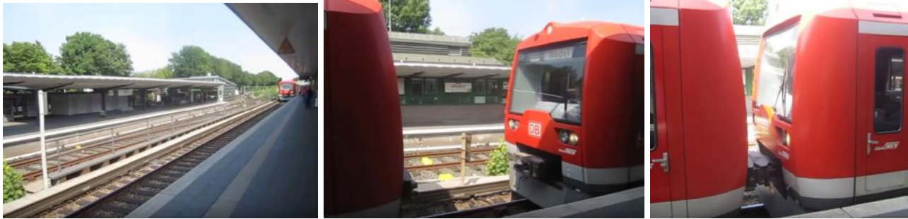
Hamburg S-Bahn docking of S1 train from Poppenbüttel onto a train from the Airport (own work)
