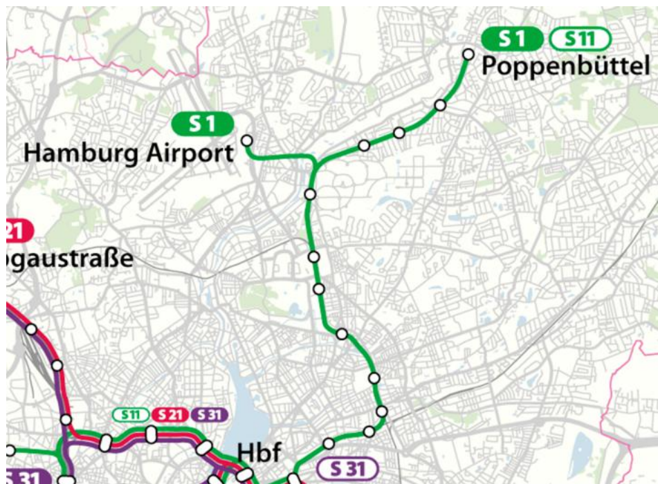
The S1 In Hamburg branches without dividing frequency by splitting trains (source: wikipedia, user NordNordWest).
