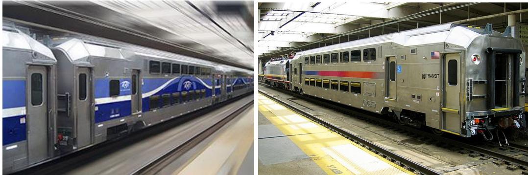
Left: AMT Bombardier multilevel car with high & low floor doors right: NJTransit Bombardier multilevel car with high & high/loor floor doors (source: Bombardier)
