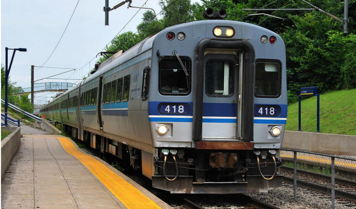
The MR-90 vehicles used on the Deux-Montagnes line. Source: wikipedia, Mtlfiredude
