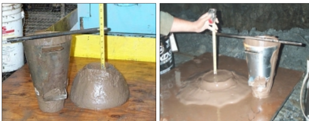
Figure 1 – Paste Slump – 175 mm (left) and 250 mm (right)
