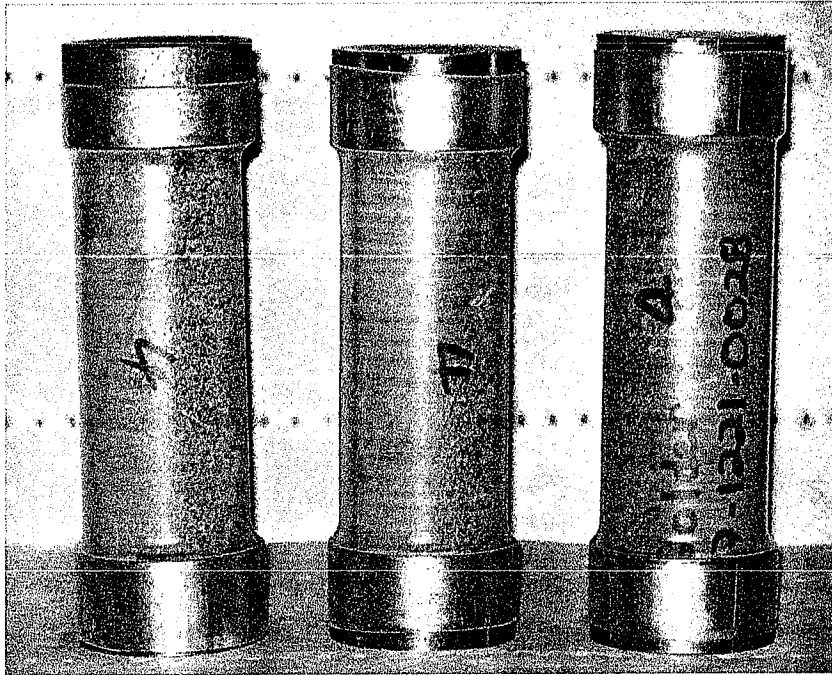
Typical Pre-Test Triaxial Confined Specimens
