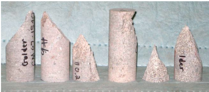
Post-Test UCS Specimens
