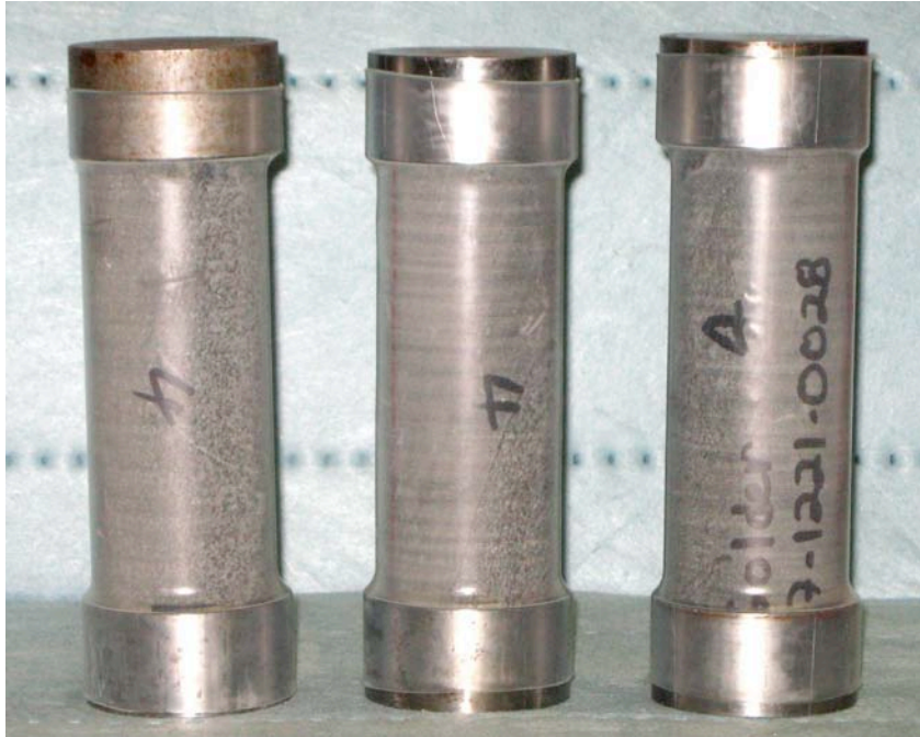
Pre-Test Triaxial Confined Specimens
