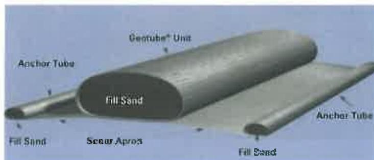
*Cross section of a Geotube<sup>®</sup> beach installation.*
