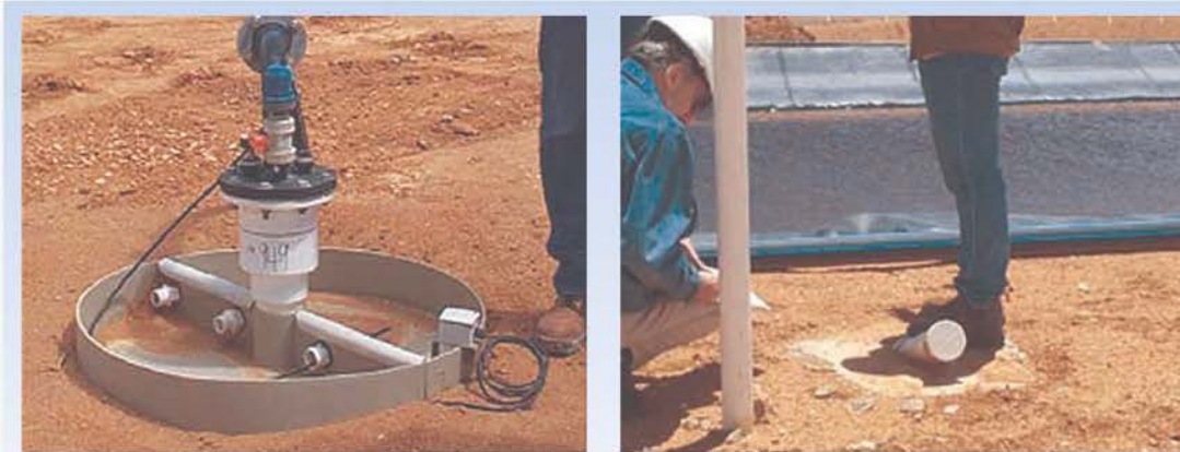
Wellhead with drip tray and online detector (left); evaporation pond with leak monitoring (right) at the Beverley ISL mine. A comprehensive environmental impact assessment (EIA) process based on a thorough understanding of local site conditions, field trials and baseline environmental data that demonstrated well field containment was required before approval to begin operations. Ongoing environmental monitoring provides assurance that the facility is operating as planned.
