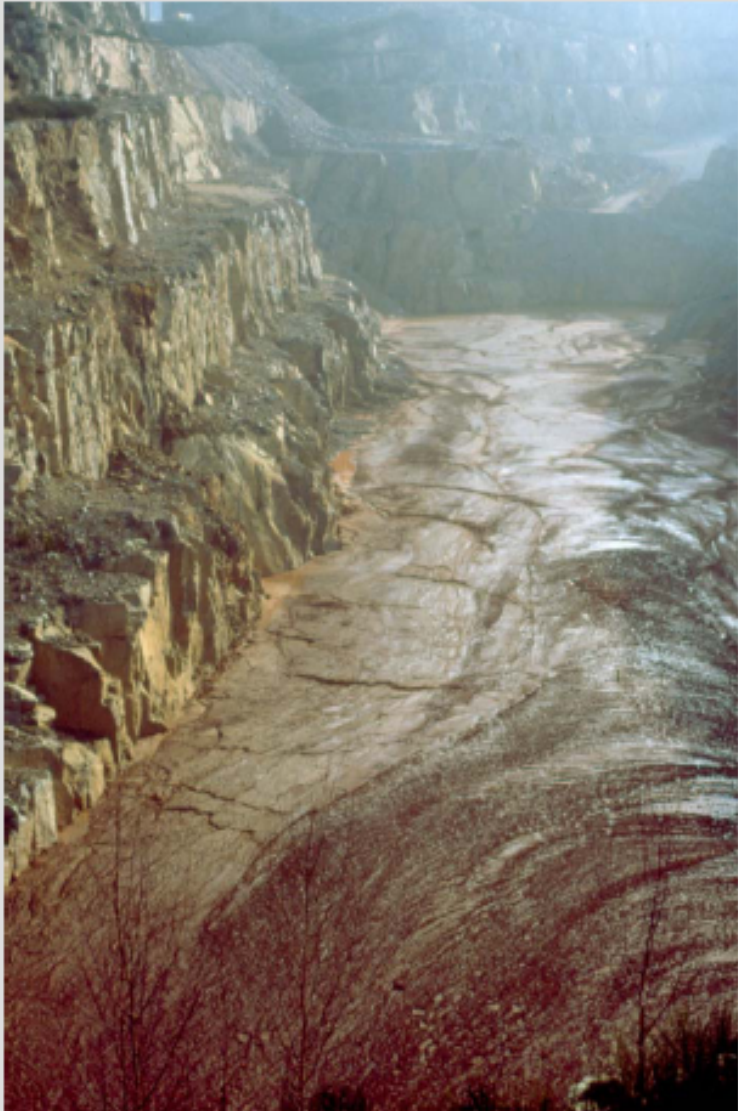
Tailings disposal in Bellezane MCO 105 open pit (Haute Vienne, France)
