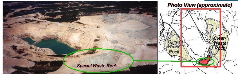
Potentially acid-generating waste rock to be backfilled into the adjacent pit – Example of McClean Lake
