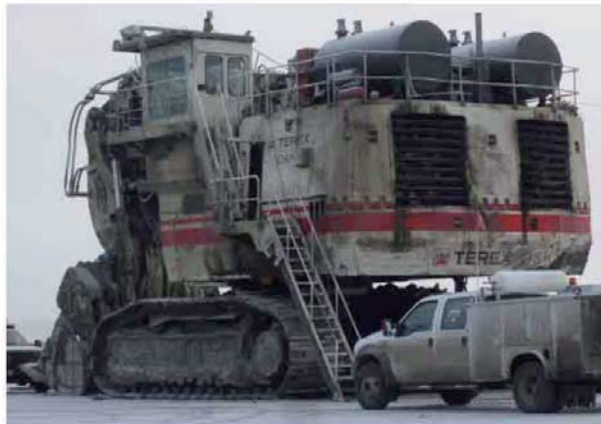
Figure 6: Terex RH200 engine exhaust silencer installation.
