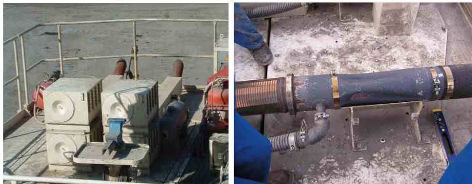
Figure 4: Engine air intake filters and exhaust venturis.
