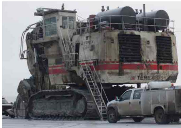
Figure 6: Terex RH200 engine exhaust silencer installation.
