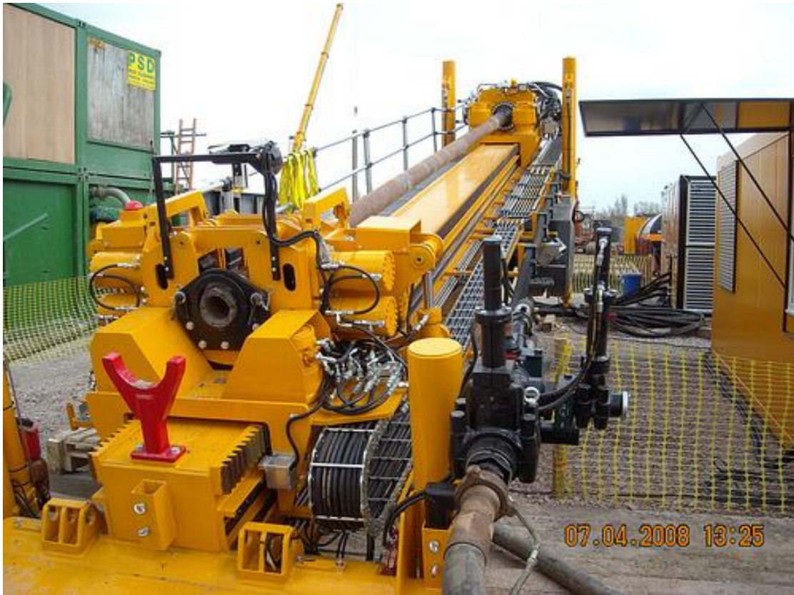
Figure 7: Photo of typical directional drilling rig
