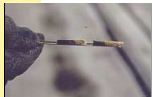
Lumber under five inches thick requires a minimum of 0.40 inch penetration; lumber over five inches thick requires a minimum of 0.50 inch penetration.
