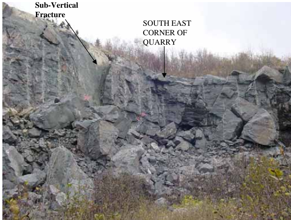
Photo 6. Area view of a sub-vertical fracture (photo looking south-east). The projection of the fracture plane separating the two massive sandstone beds continues through tank T-101 80m to the north. However, inclined borehole BH-4 and evidence from the north-east corner of the quarry cliff face (i.e., no vertical offset of the shale beds) shows proves that this fracture does not exist in the vicinity of tank T-100.
