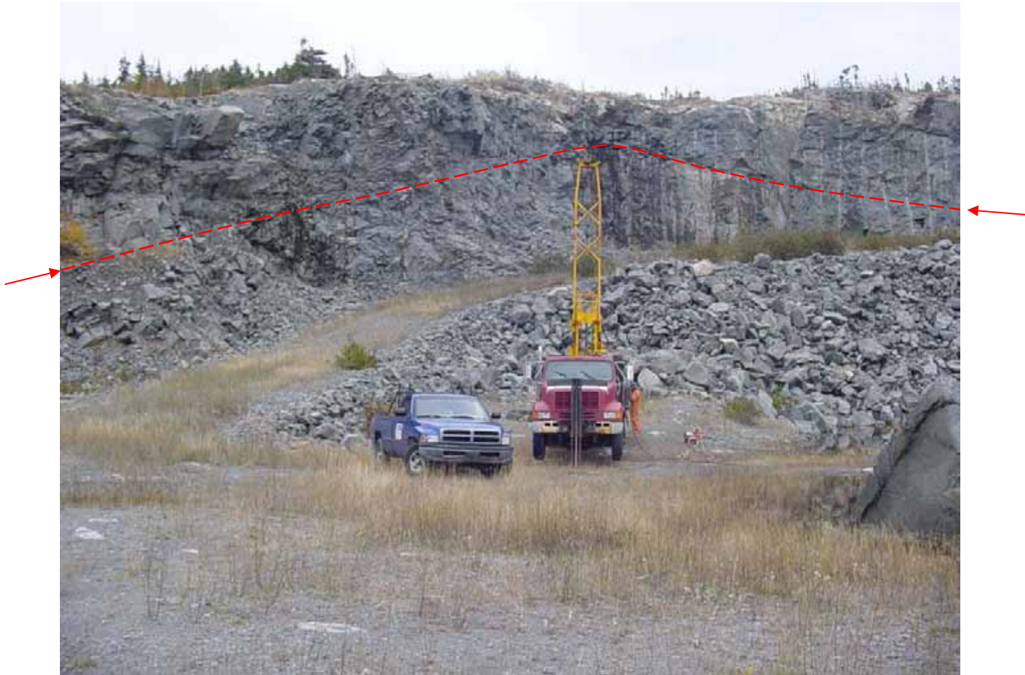
Photo 6. Rock face east of borehole BH-1 (near tank T-100). Note: No vertical offset of shale beds.
