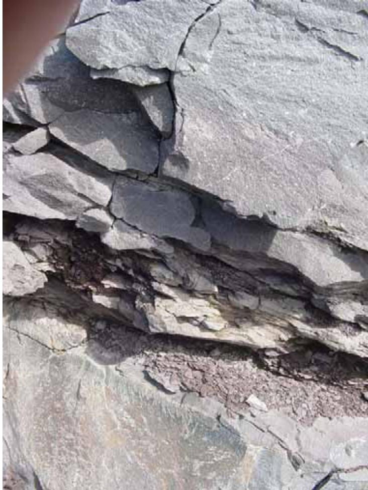
Photo 4. Green grey flaggy (thin layered) sandstone found on cliff face south of the tank locations. May be the same type of source material for ground up silt and sand found in borehole BH-2.
