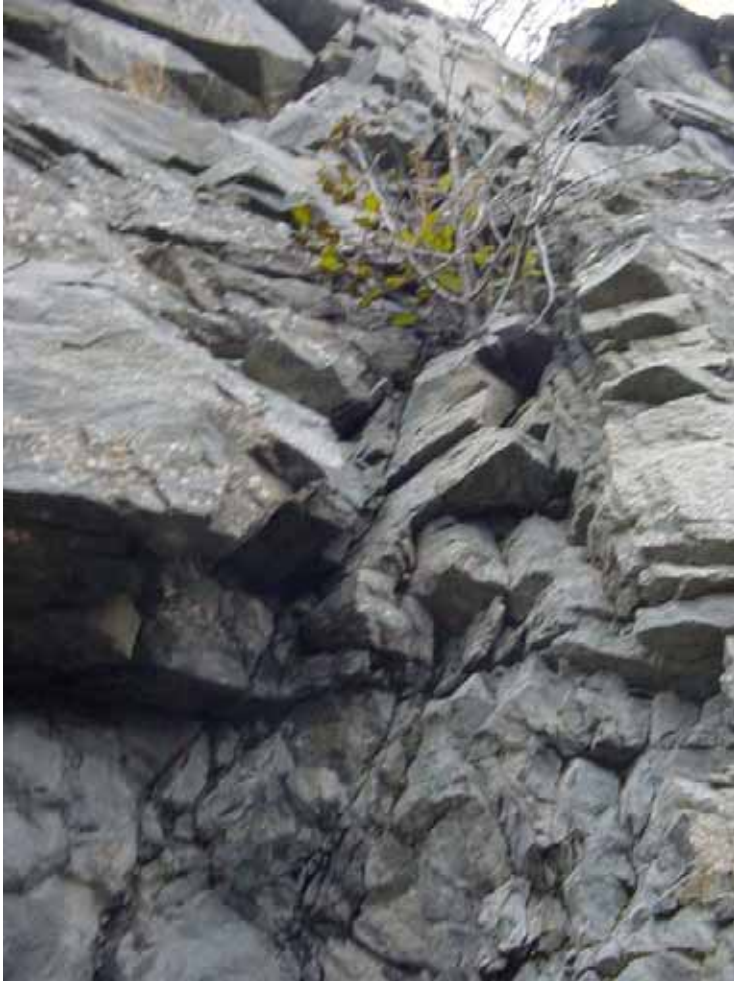
Photo 16. Close up of tight vertical jointing passing through conglomerate and sandstone layers near BH-2 (Tank T-101). Note: no vertical displacement indicating rock has not been subject to fault movement.
