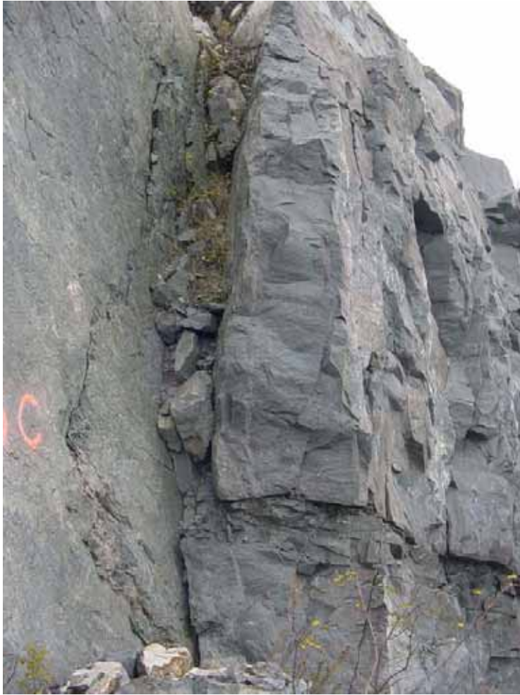
Photo 9. Close-up south cliff face of quarry. Note: sub-vertical fracture (looking south along east cliff face).
