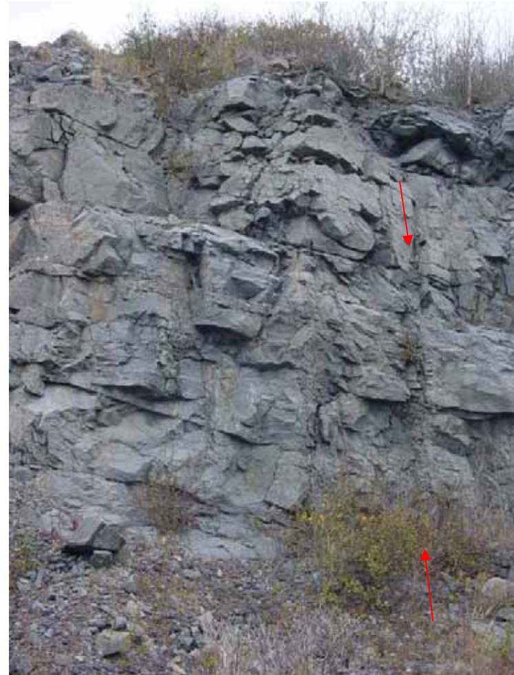
Photo 15. Close-up of formation showing jointing along bedding planes and running near perpendicular to beds. No vertical offset was observed indicating rock near tank T-101 is stable.
