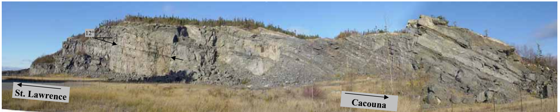
Photo 1. View of rock face on south side of quarry showing typical massive sandstone rock beds dipping at low angle (12 degrees) to the southeast
