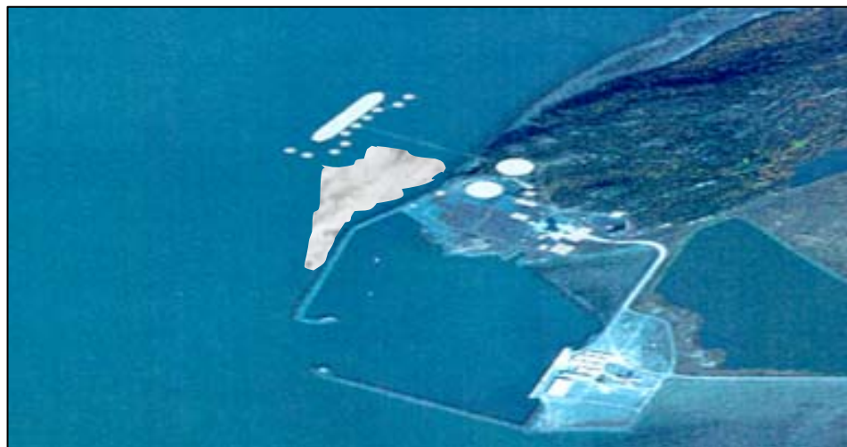
Figure 5 Schematic Illustration of Fast Ice Zone Expected to Form on the Upstream Side of the LNG Terminal
