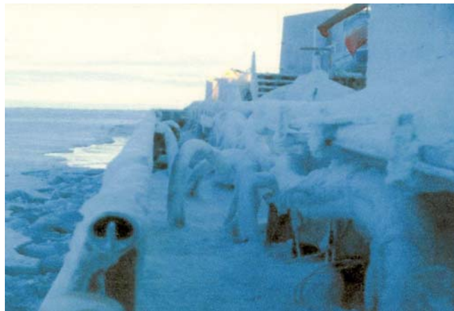
Figure 6.9: Marine icing is common in the Gulf of St. Lawrence and is a factor that can limit vessel transit speeds in light ice conditions, when air temperatures are low.
