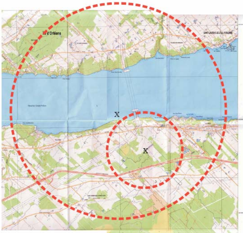
Figure 1: The thermal radiation danger zones for spills listed in Table 1. Red circles are distances to radiation intensities of 1.6 \text{ kW/m}^2 for a spill with fire; smaller for loss of primary containment of land storage tank, larger for spill from one hold of LNG tanker. X marks the spill location.
