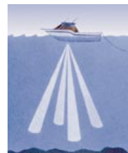
Transducer and electronics: molded composite plastic transducer head with four beams at 20° from vertical in a convex configuration, external temperature sensor, electronics assemblies, fluxgate compass, pitch and roll sensors.
