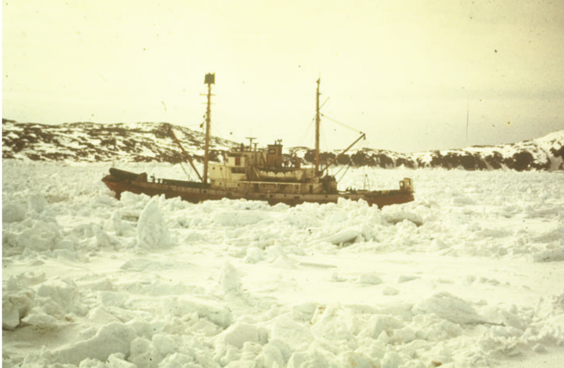
Photo 39 Small ship in thick first-year ice under pressure, Gulf of St. Lawrence in April. The Arctic Endeavour is lifted out of the water because of the pressure from the ice (archive, courtesy Canadian Ice Service)
