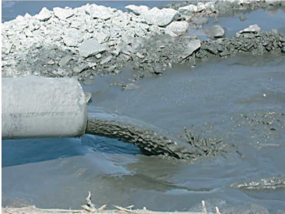
Fig. 1. Slurry of tailings discharged in a tailings impoundment.
