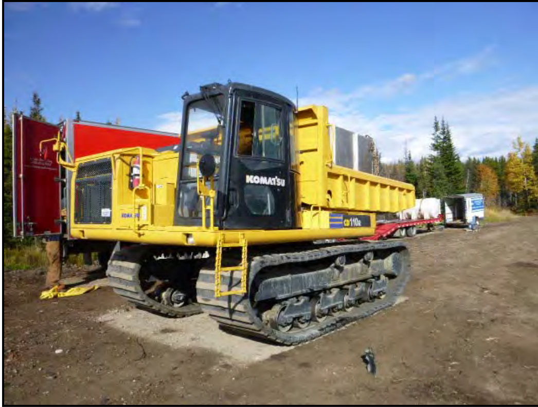
Figure 5 - Qualitas subcontractor's Komatsu CD 110R crawler
